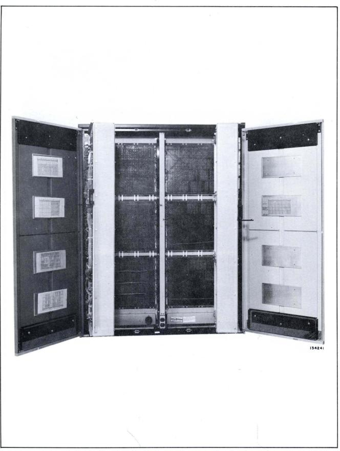
Figure 4. Interior Model 70/45 Processor (Rear View Showing Frame Opened)
